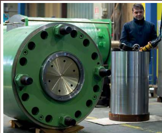
↑ Cold rolling mill 1.350 mm bore with hydraulic drive unit
